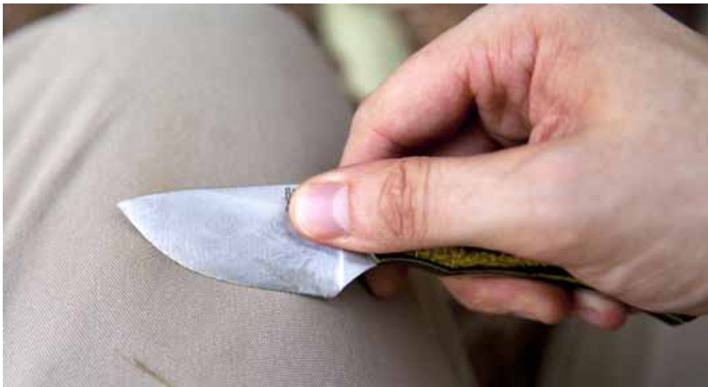
In a pinch, a pant leg can be used as a strop. Rubbing some sand, dirt, or other abrasive into the fabric can help speed up the process.
