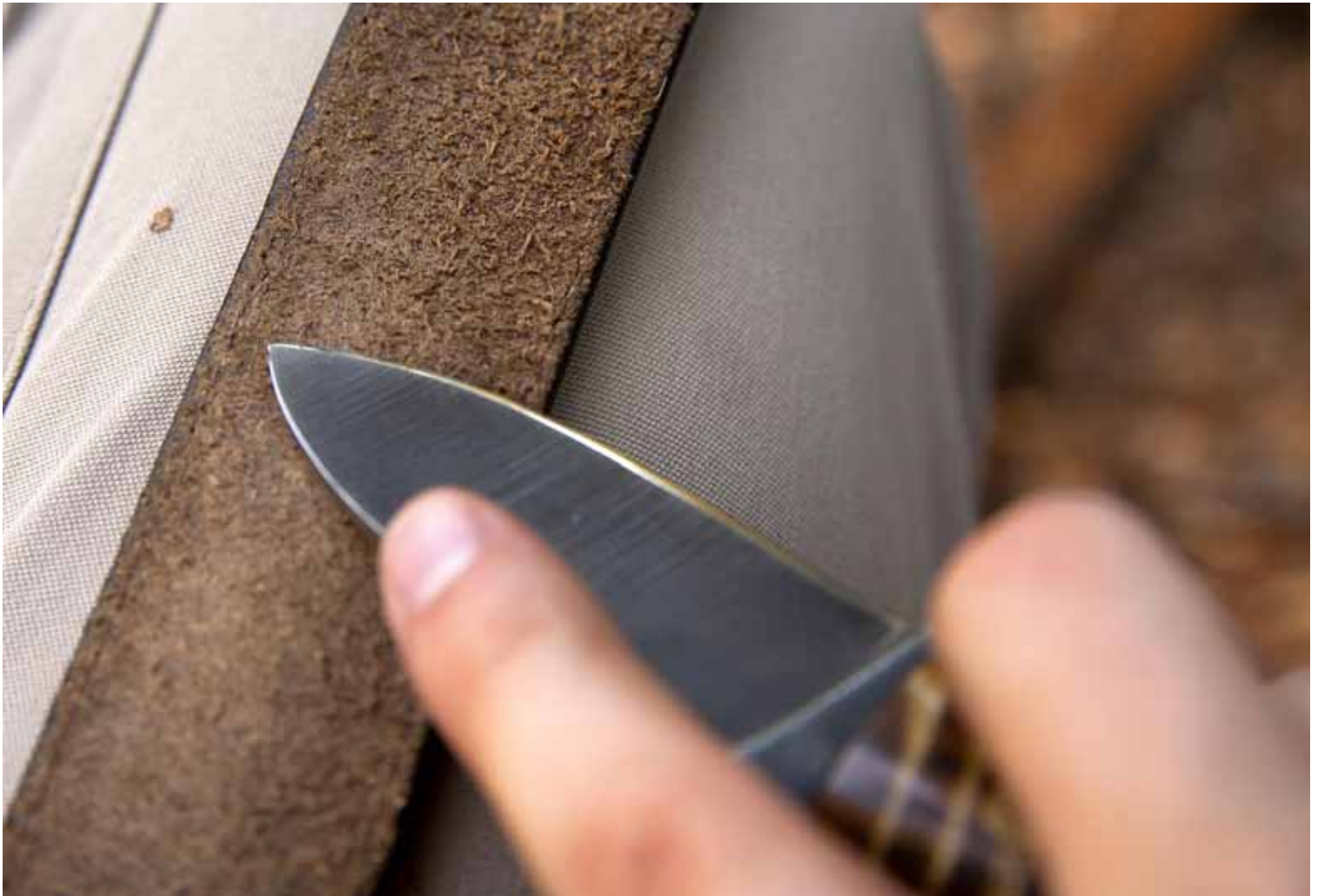
Using a stout leather belt, maintaining an edge is far easier than re-sharpening.
